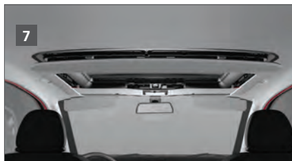
Attaching the trimshell (3) to the basic element (2) with 2 screws at the front and subsequently with 14 clips located in the trimshell.
