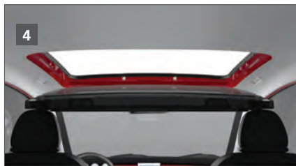
Fitting of the spoiler roof's basic element (2) into the available 2 hooks at the front of the roof frame (1).
